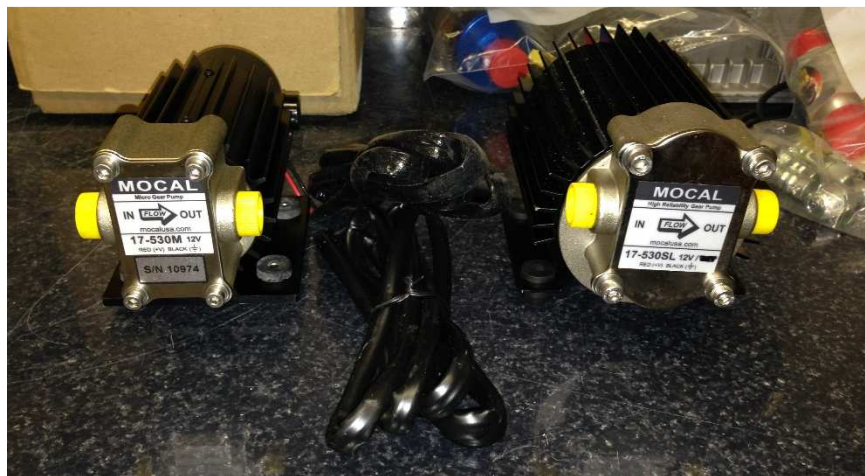
Figure 3-19. Oil feed pump on left and oil scavenge pump on right.
