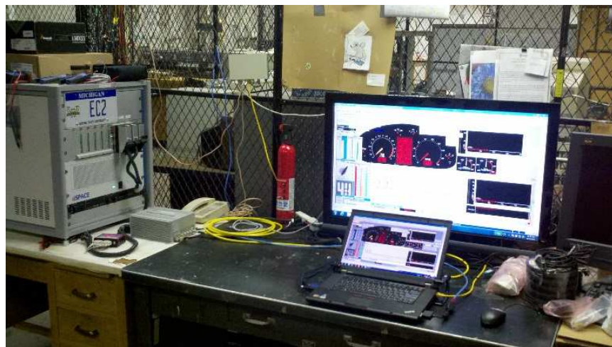
Figure 3-2. Year 2 HIL test bench.
