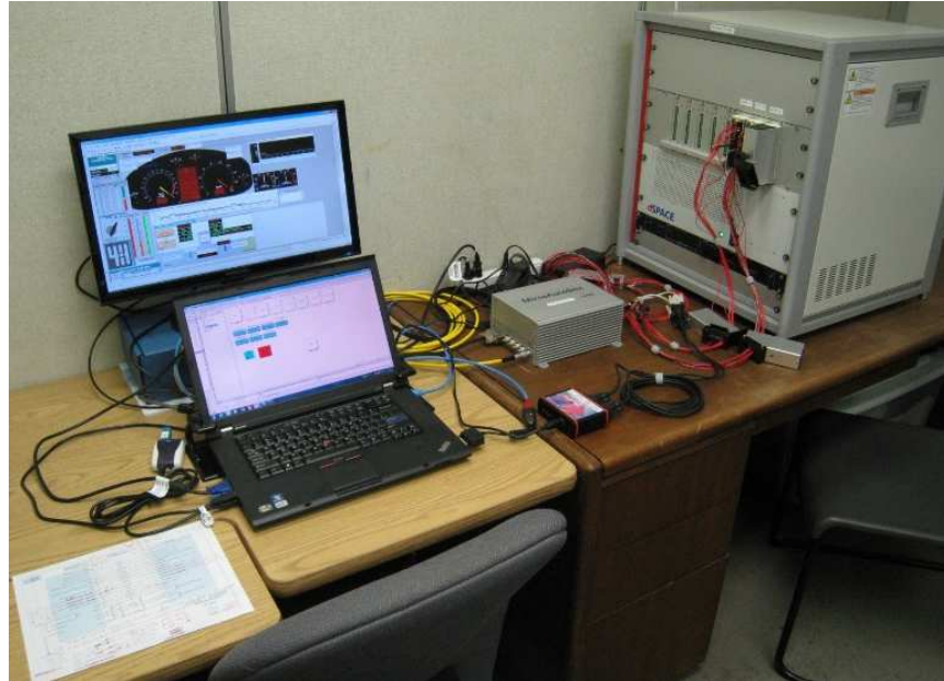
Figure 3-1. Year 1 HIL test bench.
